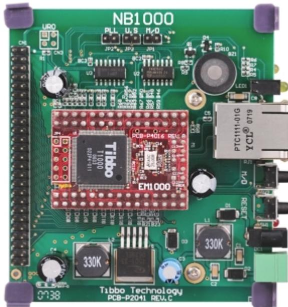
The NB1000 board is based on the [EM1000](#) embedded module.
