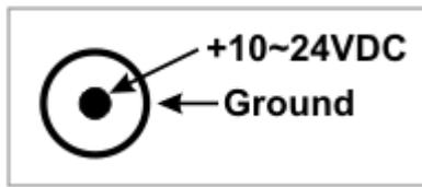
Alternatively, the DS1206N-RS can be powered through pin 9 of the DB9M (RS232) connector, while the DS1206N-TM can be powered through pin 2 of the TTL interface connector. Two internal diodes combine power jack and pin 9 (pin 2) inputs into a single line, which goes to the internal regulator of the DS1206N.
