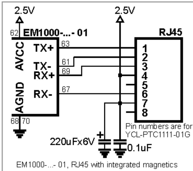
Once again, the EM1000-...-00 is a legacy part that has been replaced with the EM1000-...-01. In case you have already made the PCB based on the EM1000-...-00 specifications and are not willing to change it, you can easily modify it to accommodate the EM1000-...-01 (see diagram below):
