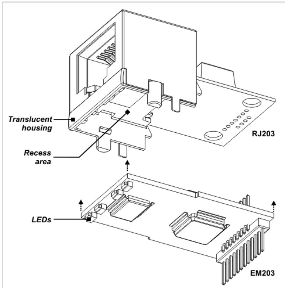
The RJ203 can also be used in combination with the EM203 Ethernet-to-serial module (documented in the "Serial-over-IP Solutions Manual") or [EM1206](#) BASIC-programmable Ethernet module.
