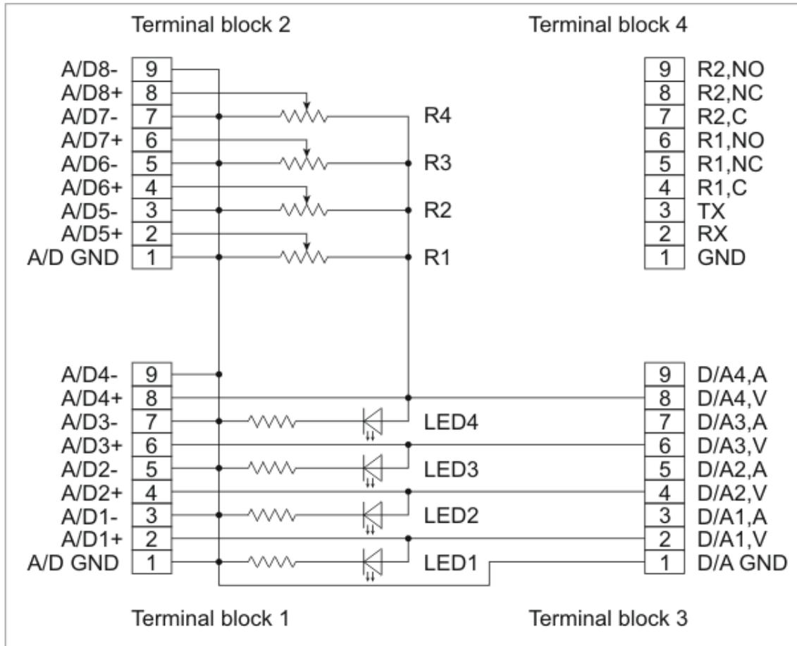
Voltage outputs of D/A channels 1-4 are connected directly to A/D inputs 1-4, and also to four red LEDs 1-4. The brightness of these LEDs is proportional to the voltage on D/A outputs. Obviously, LEDs will only work for positive output voltages and will stay off for negative voltages. Thus, LEDs provide indication only for 1/2 of the D/As' output range.
