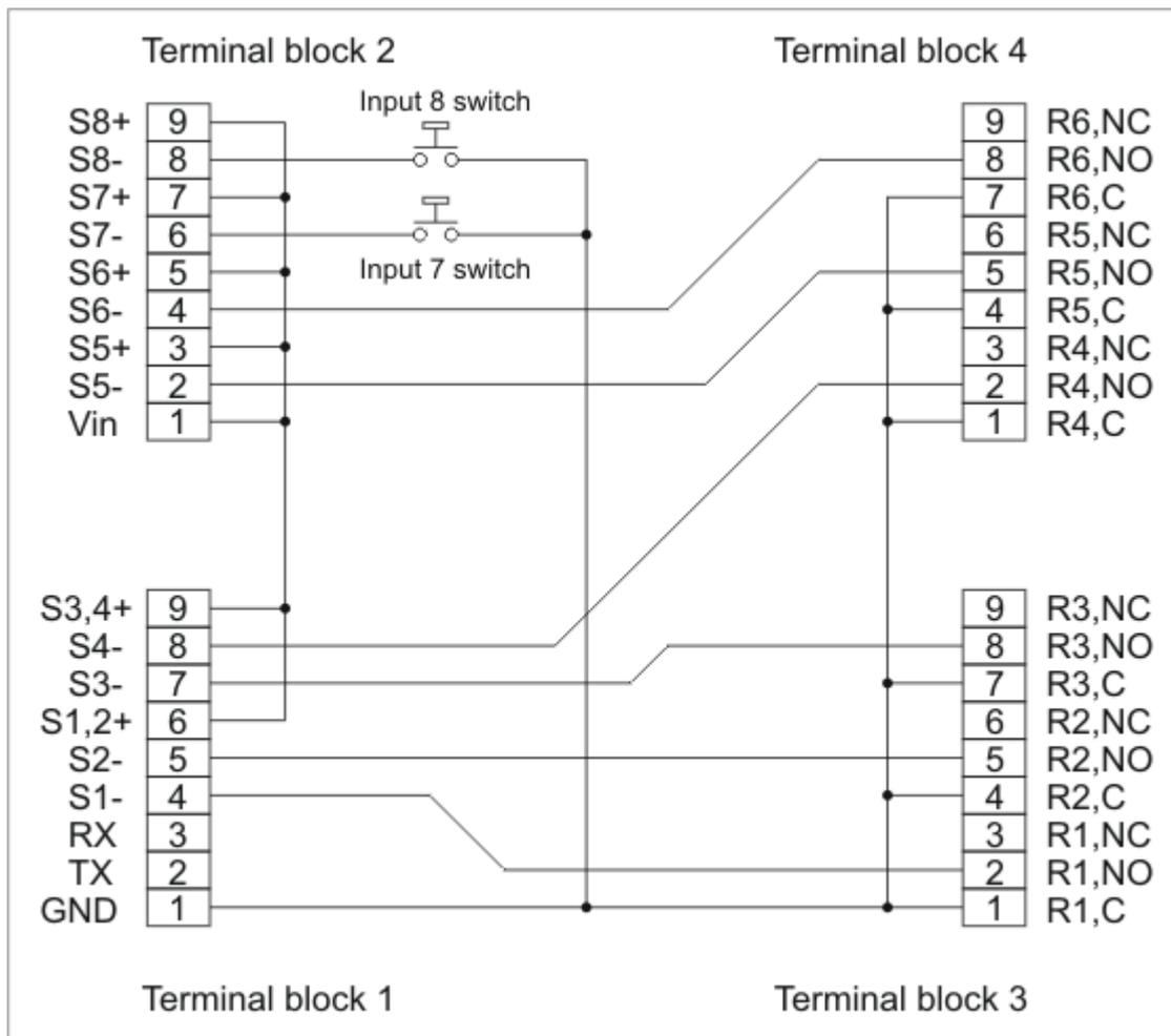
Relays 1-6 are wired into sensor inputs 1-6. They commutate "Vin", which is the voltage from the power source for the DS1005. When a relay is activated, this voltage is applied to a corresponding sensor input.
