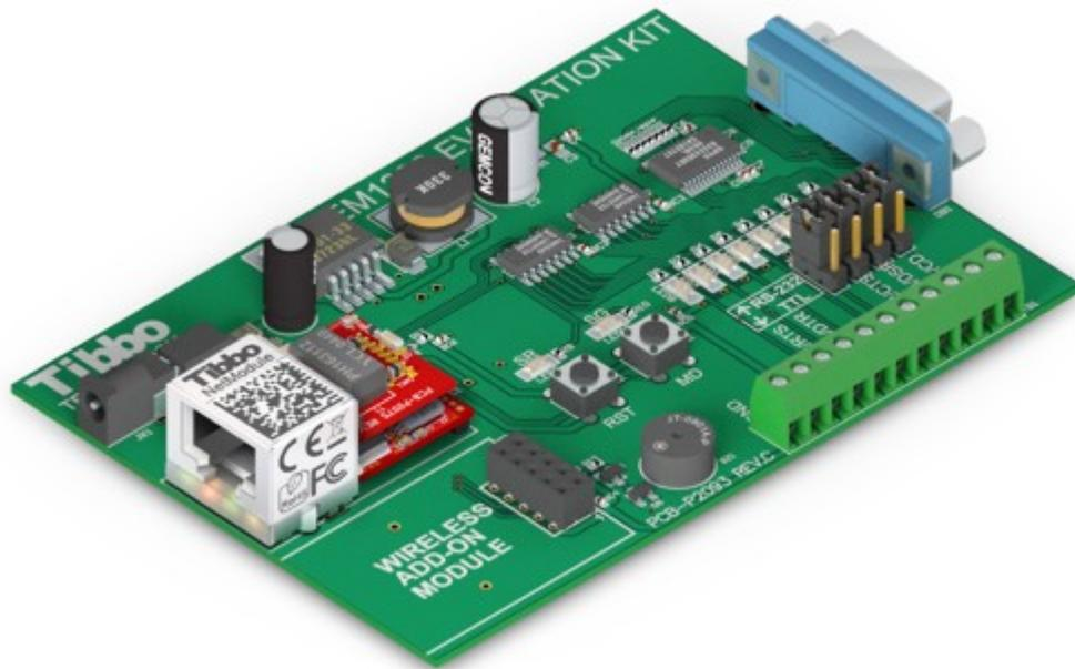
The EM1206EV Evaluation Board offers a convenient way to test the [EM1206](#) BASIC-programmable Ethernet module.
