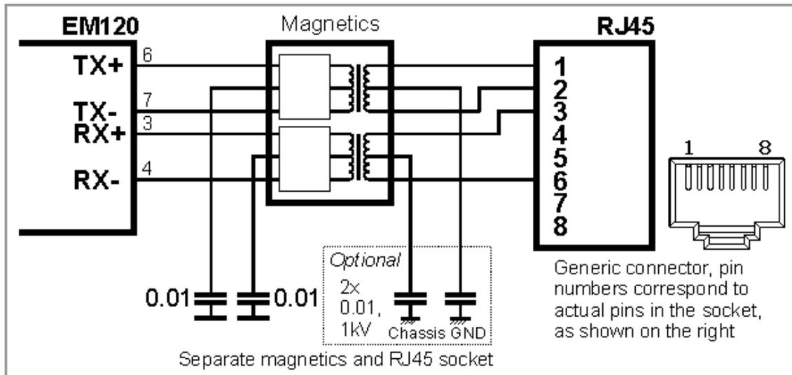
It is important to make the PCB traces connecting the Ethernet port pins of the EM120 to the magnetics circuitry as short as possible. Making the wires too long may cause the noise level generated by your PCB to surpass the maximum radiated emission limits stipulated by the FCC and CE regulations. Additionally, longer Ethernet lines on the PCB will make your board more susceptible to the ESD (electrostatic discharge) damage.
