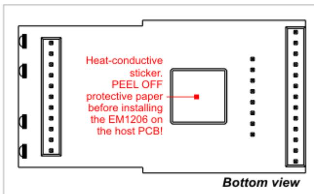
To further lower the operating temperature of the EM1206 we advise you to arrange a copper area on the host PCB and in contact with the heat-conductive sticker. Best results are achieved when the copper area is larger, and also when two copper areas are provided on both sides of the host PCB and interconnected by a number of large vias.
