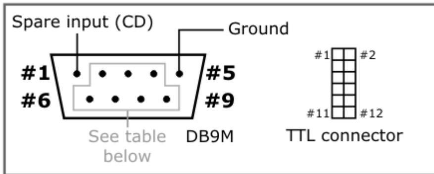
DB9M connector pin assignment:
