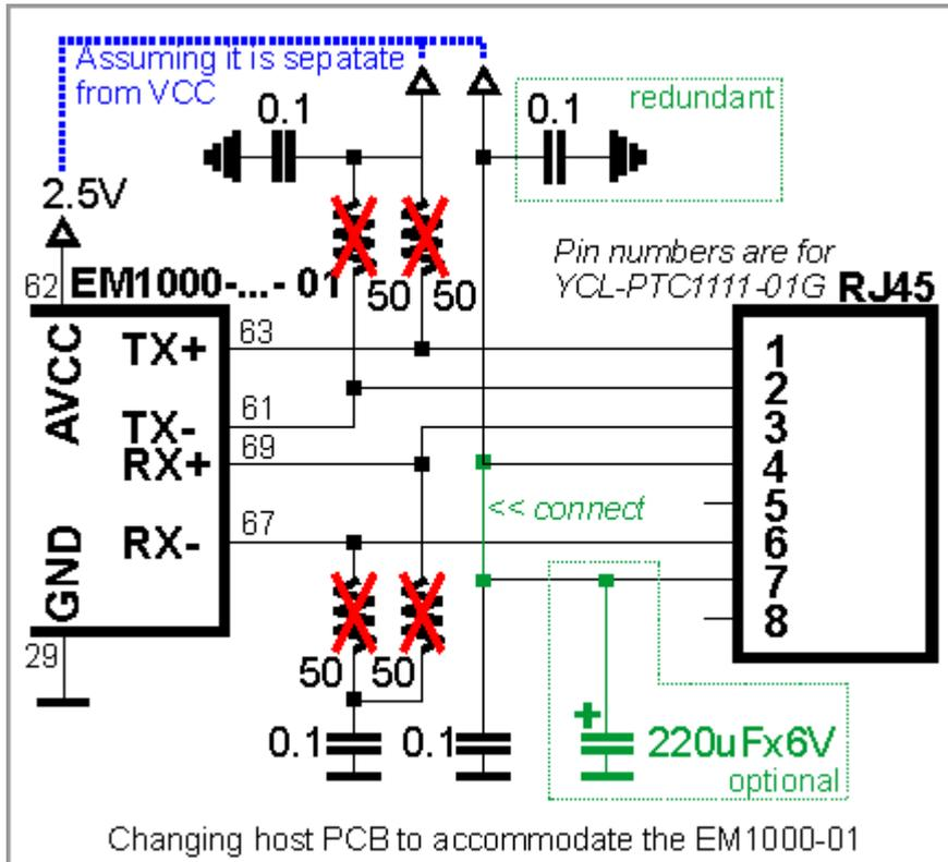
It is important to make the PCB wire connections between the Ethernet port pins of the EM1000 and external magnetics circuitry as short as possible. Making the wires too long may cause the noise level generated by your PCB to surpass the maximum radiated emission limits stipulated by FCC/CE regulations. Additionally, longer Ethernet lines on the PCB will make your board more susceptible to the damage from the ESD (electrostatic discharge).
