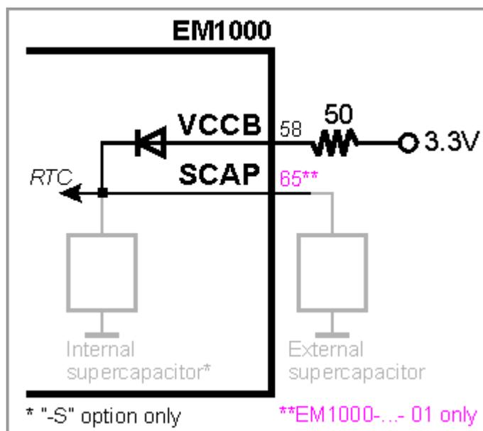
The EM1000-...-S carries the supercapacitor on the bottom side of its PCB (see [Mechanical Dimensions](#)). With this supercapacitor present, it is impossible to solder
