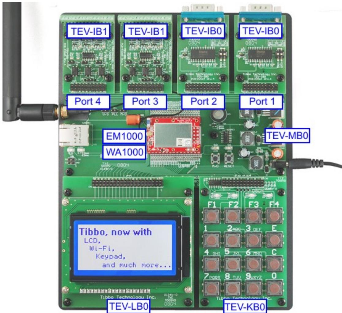
The EM1000-TEV development system has been designed to aid you in developing data terminals, data collection devices, and control equipment based on the [EM1000](#) embedded module. Hence, the abbreviation: "TEV" stands for "terminal evaluation".
