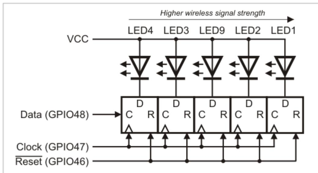
If you want to switch an LED ON then set the corresponding data line LOW. The data bit for the LED#1 (indicating the highest signal strength) is clocked in first.
