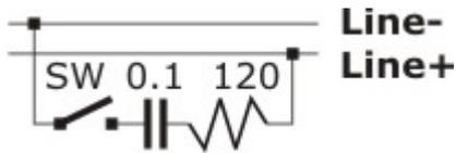
If you are using RS485 mode (SW1 and SW2 are closed) and you want to terminate the RS485 bus, then you only need to close either SW5 or SW6. Having both switches closed will effectively add two termination circuits to the same bus!
