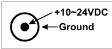
Alternatively, the DS1206 can be powered through a pin 9 of the DB9M (RS232) connector. Two internal diodes combine power jack and pin 9 inputs into a single line, which goes to the internal regulator of the DS1206.
