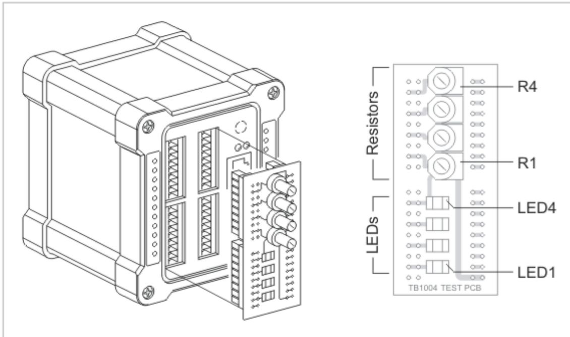
The TB1004 test board is provided for the convenience of evaluating the [DS1004](#) controller ([IB1004](#) + [SB1004](#) boards). The board is basically a loopback, feeding D/
