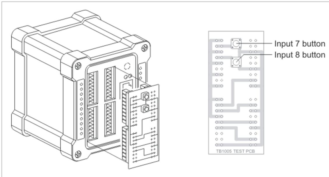
The TB1005 test board is provided for the convenience of evaluating the [DS1005](#) controller ([IB1005 + SB1005](#) boards). The board is basically a loopback, feeding relay outputs into sensor inputs of the DS1004. Schematic diagram of the test board's connections is shown below:
