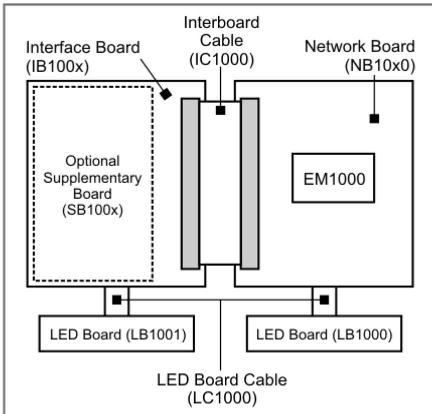
The "NB" hosts the [EM1000](#) BASIC-programmable embedded module and acts as a "connected brain" of your system. The network board carries a 3.3V switching power regulator. This 3.3V power is provided to the interface board as well.
