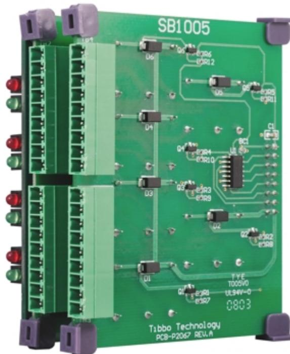
The IB1005 is the main board in the pair, and is connected to an [NB10x0](#) network board by the [IB1000](#) interboard cable. The SB1005 is a supplementary board, it exists because a single IB1005 would not be able to accommodate all required circuitry and terminal blocks. In the board pair, the IB1005 carries isolated digital inputs and the RS232/485, while the SB1005 contains all relays.
